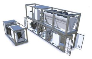
technology. The Power to Gas process is used to transform electrical energy into chemical energy bound in gases which can then be used as energy storage media or as feedstock for other industries.
