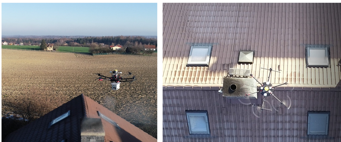
Figure 1. Transport of the Flying Laboratory using UAV before measurement (left), the position during measurement (right).
