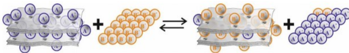
Figure 1. Scheme of cation exchange reaction principle [3].
