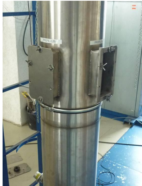
Fig. 3 Dust testing train flanges view
